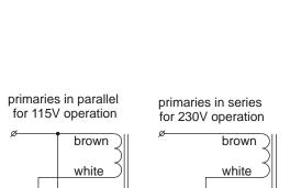
350V 0.25A yellow brown 350V 0.25A 115V white Only one tap used 6.3V 5A grey black 5V 5A 2x blue This winding is extra isolated to be 115V black connected to 500VDC 6.3V 2A violet Only one tap used at a time ! pink 5V 2A green brown orange 6.3V 2A orange yellow 6.3V 2A green/yellow striped= yellow tapescreen
